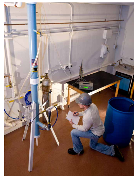
PhD student Brett Spigarelli monitors a CO 2 Scrubber designed and built by students. Their group has applied for a patent and hopes to build a pilot plant in cooperation with Carbontec Energy Corp.
