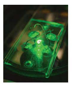
Fluorescent illumination of an microfluidic device. Wires serve as electrical contacts to manipulate cells within the microchannels.
