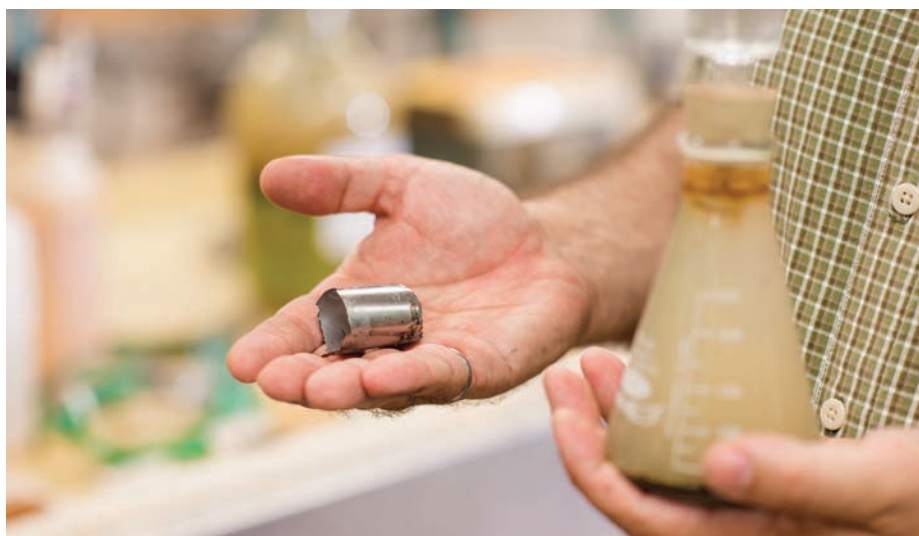
Anaerobic bacteria in the flask dissolve iron in the ferrous state. Eisele recovers it using electrolysis, producing electrolytic iron.
