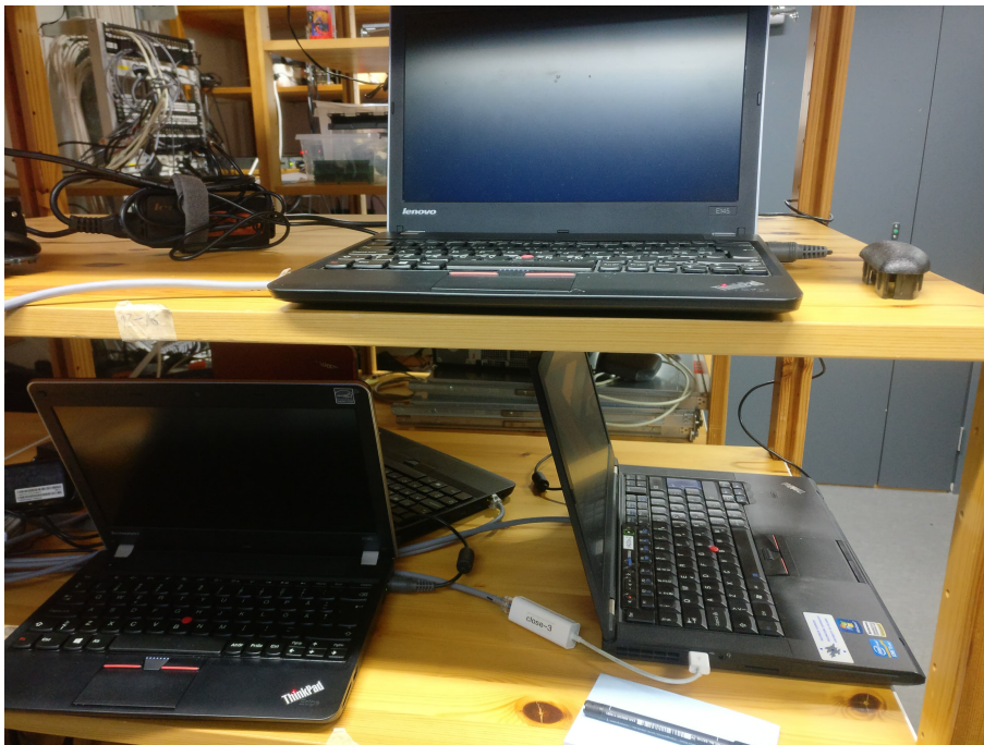
Figure 6: The actual test-bed. Master node on lower shelf on the right, slaves in the upper and lower shelf
