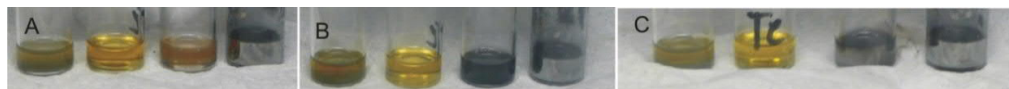
Figure 26 Reactivity of (C 6 H 13 ) 2 Te and (Et 3 Si) 2 Te with Sb(NMe 2 ) 3 and SbCl 3 . The photos show four bottles, from left to right, containing (C 6 H 13 ) 2 Te + Sb(NMe 2 ) 3 , (C 6 H 13 ) 2 Te + SbCl 3 , (Et 3 Si) 2 Te + Sb(NMe 2 ) 3 and (Et 3 Si) 2 Te + SbCl 3 . A: immediately after mixing, B: after one day, C: after three days.
