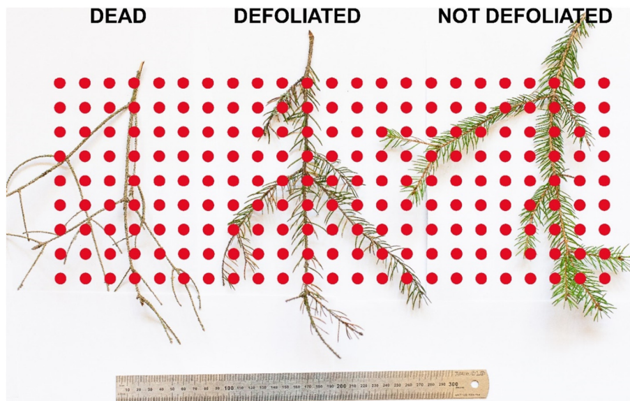
Fig. 8. Illustration of dead, defoliated, and undefoliated branches with laser-beam diameters (to scale) for a distance of 20 m using the 905 nm wavelength.
