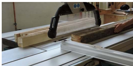
a) Processing of salvaged timber
