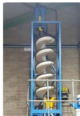
b) Spiral separation column
