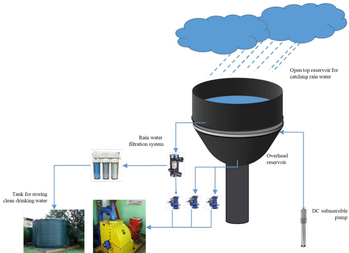
Figure 5. Rain water harvesting system
