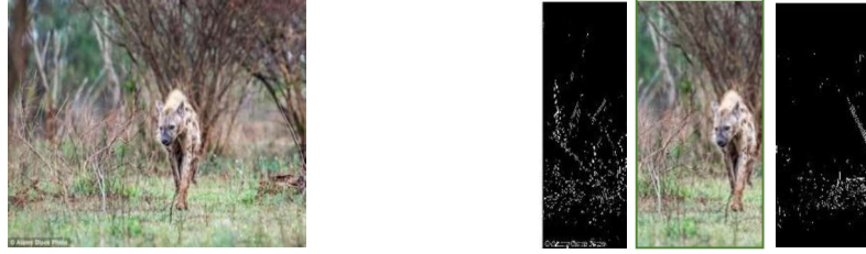
(a) Sample input image (b) Final image sent to VSN (CSR+Sobel of non-DOR) Fig. 8. Compressed significant region with edge information of the non-DOR.
