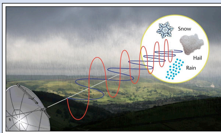
Figure 3. Schematic of dual polarisation measurement (Source: Darlington et al. , 2016)
