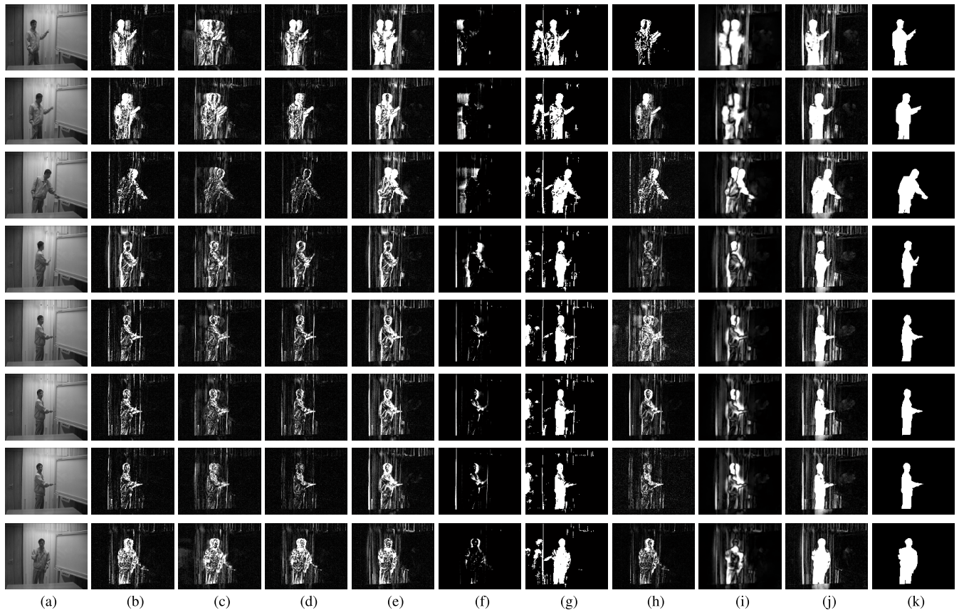
FIGURE 5. Visual results comparison on Curtain frames with dynamic background. The first and the last columns show the original frames and the corresponding annotated groundtruth foregrounds. The second to tenth columns show the foregrounds extracted by different methods in real data. (a) Original. (b) MoG-RPCA. (c) MoG. (d) RegL1ALM. (e) RPCA. (f) incPCP. (g) MEDRoP. (h) ReProcs. (i) TVRPCA. (j) TR1-RPCA. (k) Ground truth.
