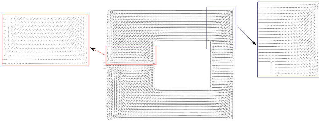
Figure 20. Director orientations in the simulation of the filling of Mold A . Inlet cross-section = 0.003m.
