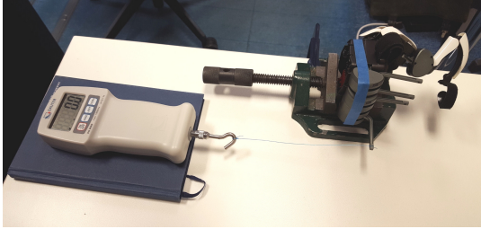
Fig. 7. Measuring the torque of a Dexmo finger driver. The attachment point is 50 mm from the pivot.
