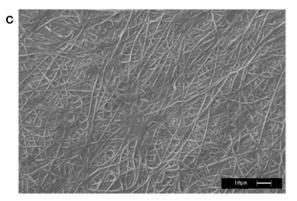
**FIGURE 2** | Representative SEM images of PLLA mat **(A)**, mHELP deposited on the PLLA matrix in the absence of cross-linking **(B)** and mHELP undergone cross-linking after deposition on PLLA matrix **(C)**. Bar is  $10\,\mu m$ .
