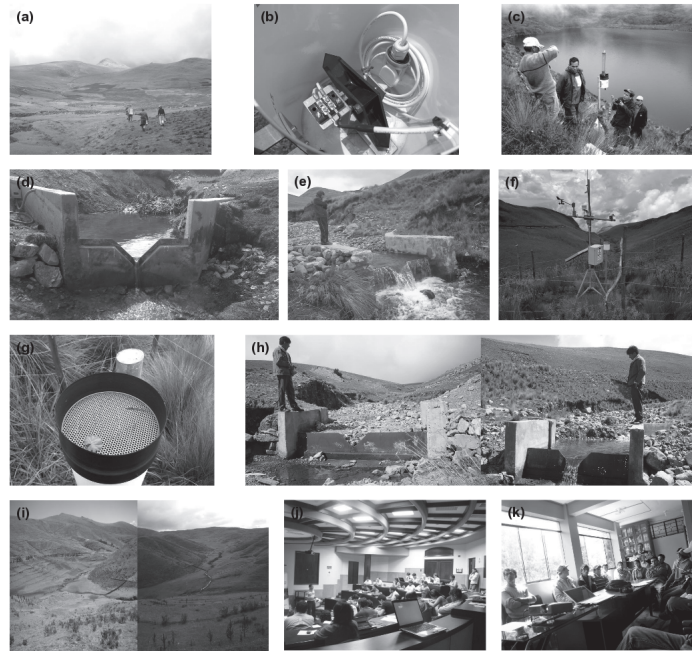
Fig. 6.25. Pictures of equipment and catchments in the iMHEA network: (a) Selection of monitoring catchments in Tambobamba, Peru, by a group of hydrologists, local partners and users of land and water. Photo: Boris Ochoa-Tocachi, 2011. (b) Example of a tipping bucket rain gauge with a resolution of 0.2 mm installed in Lloa, Ecuador. Photo: BOT, 2014. (c) Local partners of iMHEA installing a rain gauge in Piura, Peru. The rain gauge accuracy is revised using static and dynamic calibration methods on a regular basis. Photo: BOT, 2012. (d) A weir located at the outlet of an iMHEA catchment in Ica, Peru. The V-shaped section of the weir allows an accurate monitoring of low flows. Photo: Junior Gil-Rios, 2015. (e) A weir located at the outlet of an iMHEA catchment in Huaraz, Peru. The composite triangular-rectangular section allows the monitoring of high flows. Photo: JGR, 2014. (f) A weather station is located at a central location between the iMHEA catchments in Lloa, Ecuador. The monitoring of several climatic variables, in this case temperature, relative humidity, solar radiation, wind velocity and direction and rainfall, allows for a more accurate calculation of evapotranspiration. Photo: BOT, 2014. (g) Example of a tipping bucket rain gauge in Lloa, Ecuador, with some litter retained in the filter. Photo: BOT, 2014. (h) Hydrological monitoring of two catchments under different levels of conservation/alteration in Cochabamba, Bolivia. A local farmer contrasts visually (left) a highly degraded catchment produced by cultivation and overgrazing, against (right) a relatively conserved catchment situated closely to the former. In what we refer to as the 'Placebo iMHEA effect', local users recognize the relevance of monitoring impacts, even before seeing any data. This has supported the implementation of new monitoring sites and the implementation of water conservations practices more smoothly. Photos: Luis Acosta, 2012. (i) Highly seasonal catchment in Tambobamba, Peru. In puna, the landscape is markedly different during the (left) dry season and the (right) rain season. Photos: BOT, 2012, 2013. (j) An International Course on Andean Hydrology and Hydrological Monitoring organized by Nature and Culture International, CONDESAN, the University of Piura, Peru, and iMHEA in Piura in 2013. Photo: BOT, 2013. (k) A group of farmers in a meeting with local decision makers and hydrologists from iMHEA in Pacaipampa, Peru. Photo: BOT, 2012.
