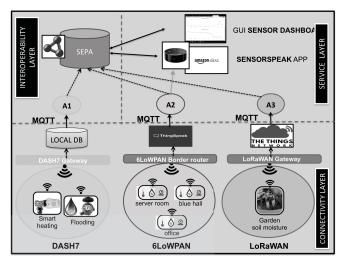
Fig. 2. The concrete IoT architecture currently implemented at ARCES@UNIBO
