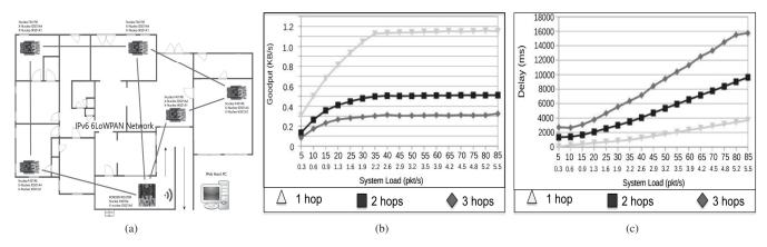
Fig. 3. The 6LoWPAN installation is depicted in Figure 3(a). Average network Goodput and Delay for different hop length and traffic loads are reported in Figure 3(b) and Figure 3(c), respectively
