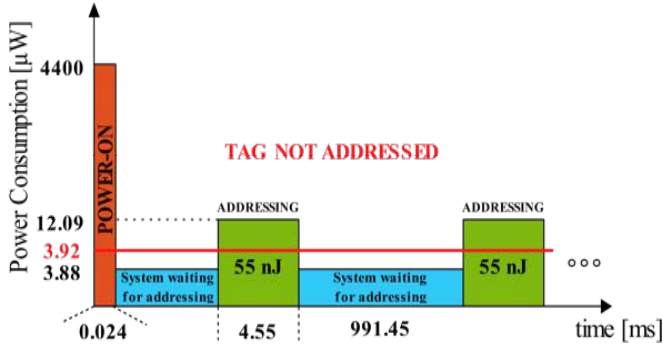
Fig. 5. Power and energy consumption of addressed tags at an activation rate of 1 Hz.
