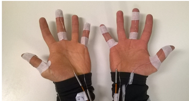
Figure 2. Location of the thermocouples for the measurements of finger tips temperature.
