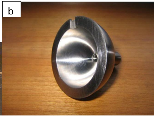
Figure 11 a) Wingbox rib of an A380 airplane and b) TiAl6V4 orthopaedic implant.
