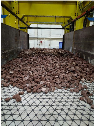
Fig. 6. Geogrid placed at the interface between the ballast and the substructure.
