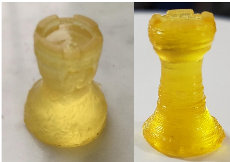
Figure 8. Objects printed with linseed oil based resin. Left: neat linseed epoxide (112 layers, 0.2 mm each, 90 s exposure time for each layer), right: linseed epoxide with 20% tri(ethylene glycol) divinyl ether (102 layers, 0.2 mm each, 60 s exposure time for each layer).
