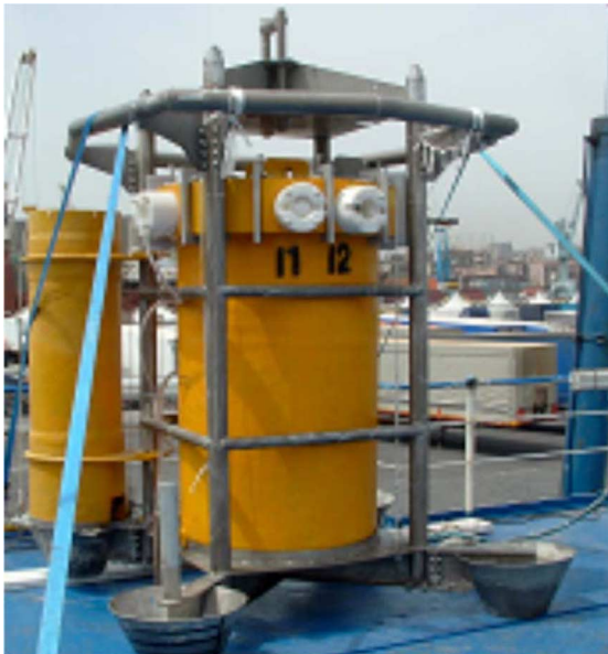
Fig. 13. The JB, deployed at TSS, is connected to the frame, and it provides several electro-optical connections for deep-sea experiments.
