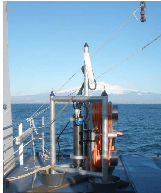
Fig. 9. The deep-sea frame (about 2.5 m high) holding the refurbished O/DE station ready for deployment.
