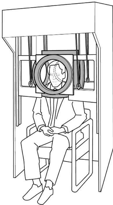
Figure 1. An example of device for sinusoidal magnetic stimulation. The exposure system consists of six Helmholtz coils in three orthogonal directions forming a cubic structure. Modified from Crasson et al. [19].
