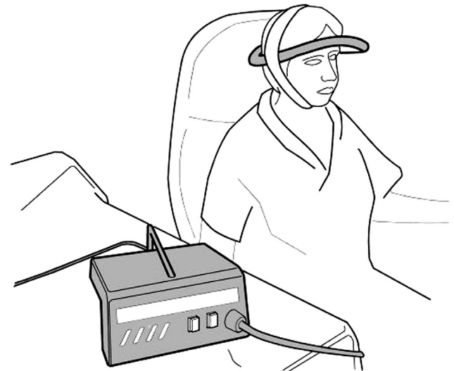
Figure 2. Exposure system used to evaluate the effect of PEMF on cortical excitability. The custom coil wrapped around (1400 turns of copper wire, 0.2 mm) a flexible plastic support is positioned to orient the positive pole of the magnetic field toward the top of the skull and connected to the pulse generator (B-01; IGEA, Carpi, Italy). Modified from Capone et al. [25].
