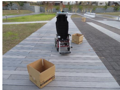
Fig.8 Wheelchair robot avoids obstacles while being navigated along the specified path.
