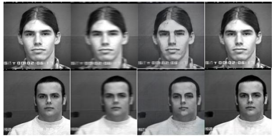
Figure 7. Shows the original image, the degraded image and the results of recover image by using our cGAN-based solution and DeblurGansin single motion blur with kernel size (20,20).
