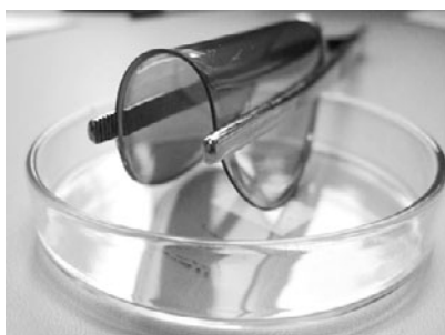
Figure 3. Picture of the film POMTETA obtained by crosslinking the OEGDG with MA using TETA as a curing catalyst.
