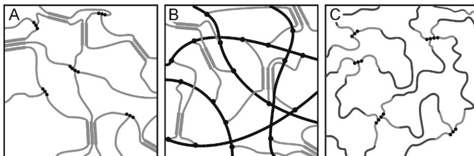
Figure 1. Scheme of network structures. (A) Networks from oligo[ \epsilon -caprolactone]- co -glycolide] dimethacrylate precursors [N-CG( \chi_G )- \bar{M}_n ], where \epsilon -caprolactone can crystallize depending on \chi_G . Modified figure reproduced with permission, [36] copyright 2010, Elsevier. (B) Networks from oligo[ \epsilon -caprolactone]- co -glycolide] dimethacrylate precursors copolymerized with n -butyl acrylate to AB networks [AB-CG( \chi_G )- \bar{M}_n ]. Modified figure reproduced with permission, [29] copyright 2010, Wiley-VCH Verlag GmbH & Co. KGaA. (C) Networks from poly( rac -lactide)- block -poly(propylene glycol)- block -poly( rac -lactide) triblock precursors with short poly( rac -lactide) blocks. The polymer networks contain: (co)oligoester segments (—), which in some cases can crystallize (==), covalent netpoints (●) from photocrosslinking by acrylate chemistry, poly( n -butylacrylate) segments (—), and/or PPG segments (—).
