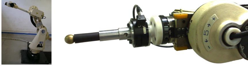
Fig. 22.2 The COMAU SMART3-S2 robot and the force sensor with its tip
