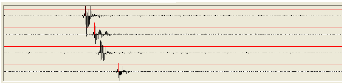
Figure 10: A click received on the 4 hydrophones. Waveform display (x-axis 9.6msec) shows a time length of 300microsec matching well with Cuvier's beaked whales' click structure.
