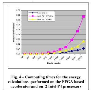
evaluation of the energy due to particle interactions, the architecture implemented onto the FPGA is mainly dedicated to that portion of the program.
