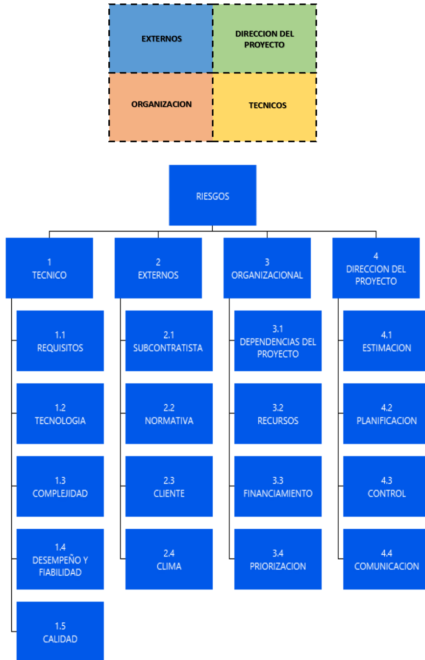
Figura 27. Risk Breakdown Structure –RiBS.
