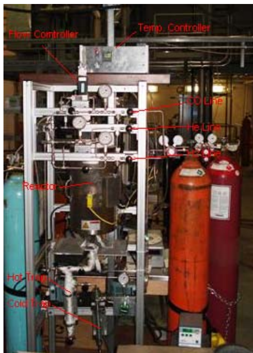
Figure C2 Front view of the fixed bed reactor for Fischer-Tropsch synthesis
