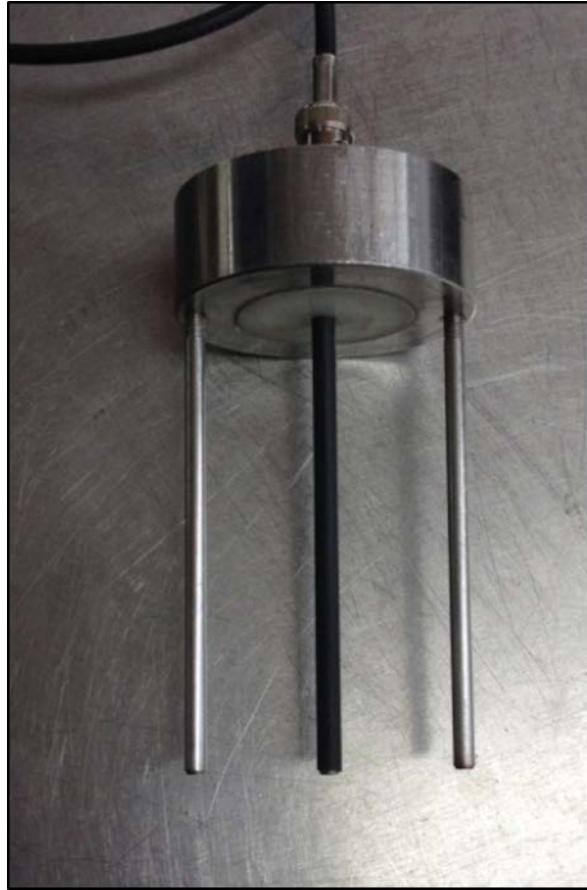
Figure 3.4 – Conventional three-rod probe. Sheathed variation shown (central rod sheathed).
