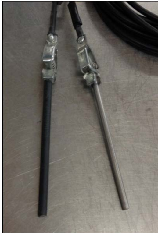
Figure 3.3 – Conventional two-rod probe. Sheathed rod on left, unsheathed on right.
