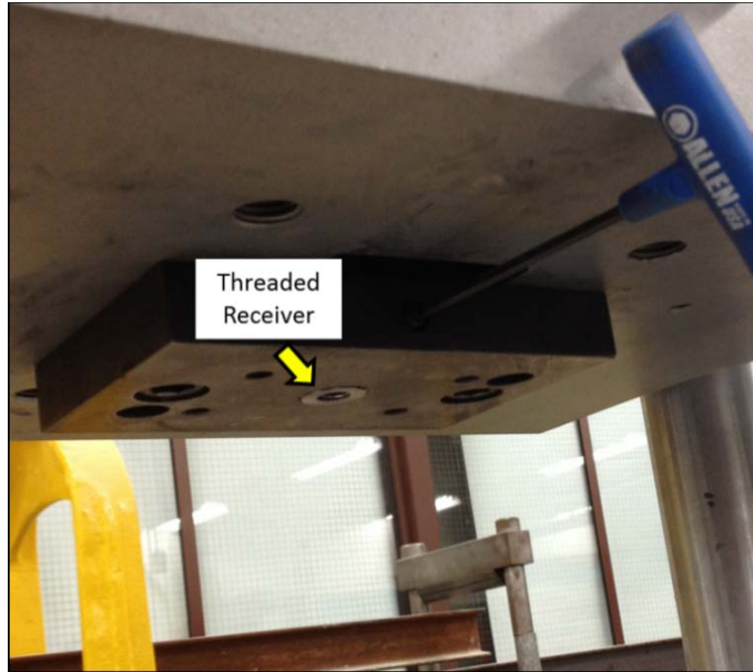
Figure 3.9 – Threaded receiver secured in place with Allen screw.
