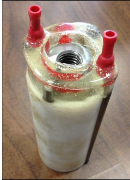
Figure 3.20 – D2 probe modified for push-test with epoxy ring and sleeve-style crimp fittings.
