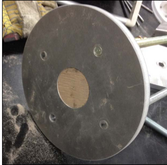
Figure 3.11 – Bottom of compaction plate with wooden plug to close access hole for conventional probe testing.
