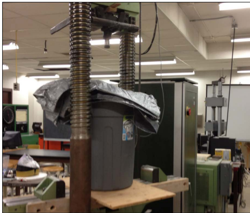
Figure 3.18 – Hydraulic press and tarp-covered plastic garbage container used for push-test.
