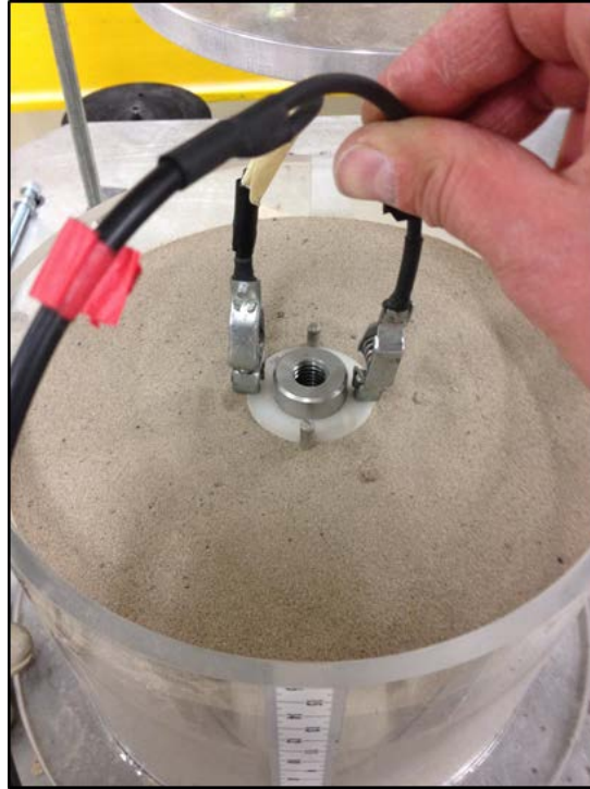
Figure 3.6 – Typical two-rod connection on Delrin® prototype.
