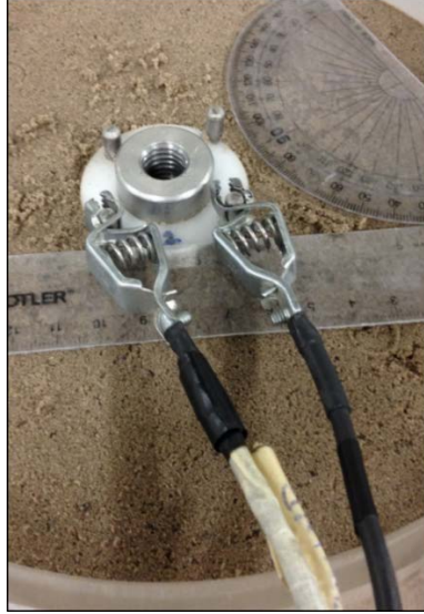
Figure 3.15 – Closely-spaced two-rod horizontally-oriented connection on Delrin® prototype.
