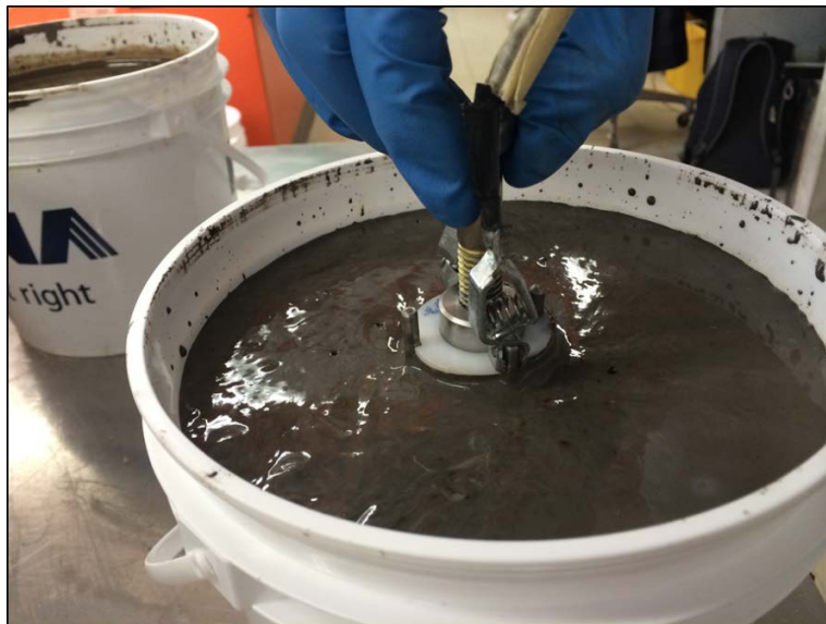
Figure 3.17 – Insertion of Delrin® prototype probe into FFT. Note nitrile glove holding bolt to prevent electrical interference in the reading.
