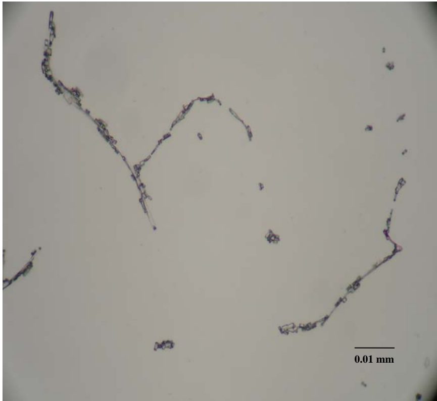
Fig. 4.10 Micrograph of fungi from thin stillage taken at a magnification of 400X.
