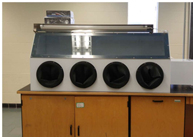
Figure 3.9. The N 2 filled glovebox used in this work.
