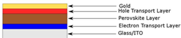
Figure 2.1. A device structure of \text{CH}_3\text{NH}_3\text{PbI}_3 -based PSC.
