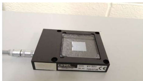
Figure 3.14. A Newport 91150V silicon reference cell.
