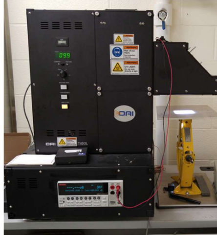
Figure 3.15. The OAI solar simulator with built-in Keithley 2420 SMU used in this work.
