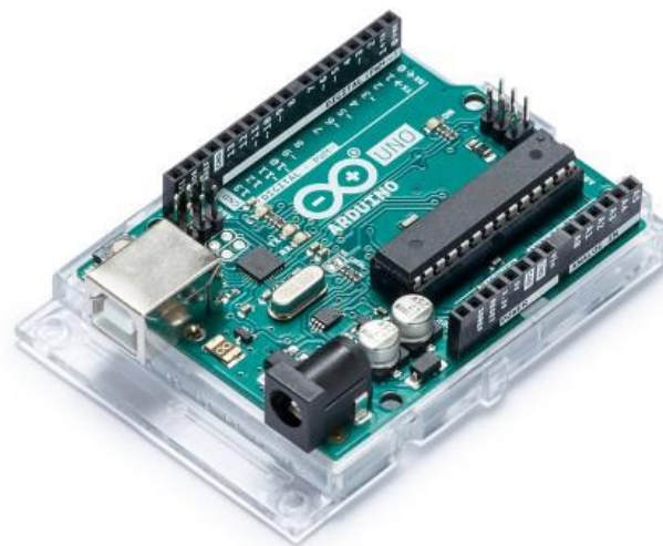
Figure 3-4: A picture of Arduino Uno Rev3 (picture source: https://www.arduino.cc )
