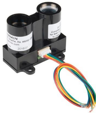
Figure 3-2: LiDAR-Lite v3 by Garmin Inc. (picture source: https://www.sparkfun.com )
