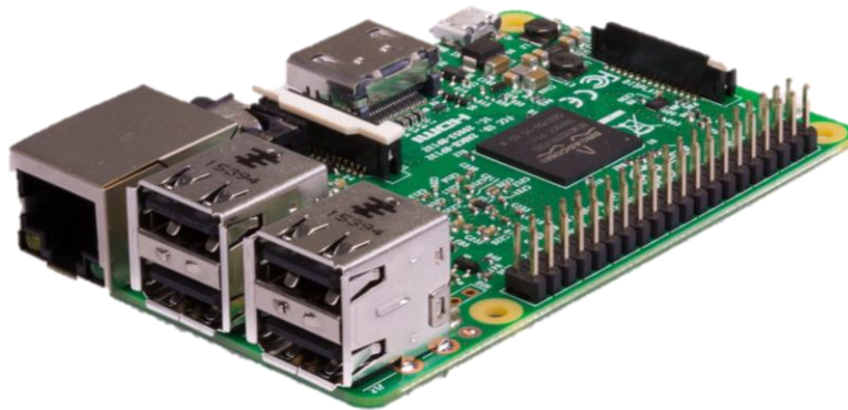
Figure 3-5: A picture showing raspberry pi 3 model B (source: www.raspberrypi.org )
