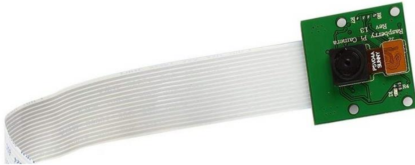
Figure 3-6: An image showing pi camera module rev1.3 (source: www.amazon.ca )
