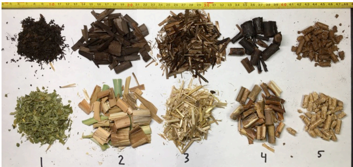
Figure A.4.3: Photograph comparing five biomass, before and after torrefaction in CTU pilot plant. From left 1. Moringa leaf, 2. Cattail ( typha spp. ) 3. Wheat Straw 4. Coppice willow. 5. Spruce pellets
