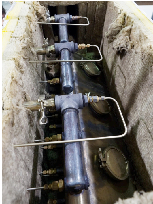
Figure A.3.14: Photograph of CTU pilot plant: Stage 2 manifold and auger shell.
