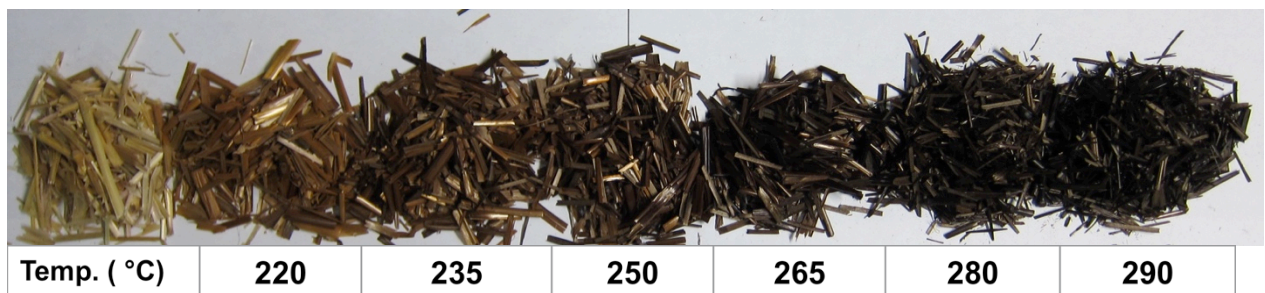
Figure A.6.3: Raw and continuous torrefied wheat straw samples, peak temperature indicated. 8.6 minutes residence time.
