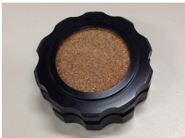
Figure 6.3: Agilent (USA) 40 mm quartz window sample powder cell loaded with mild char sample.
