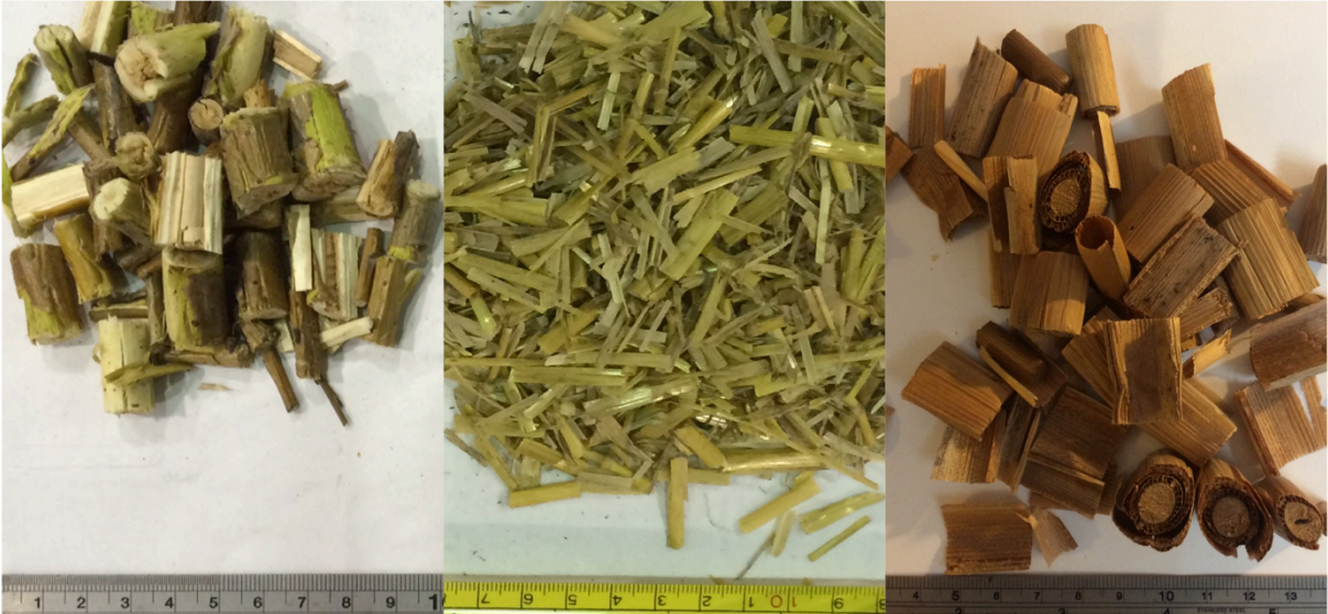
Figure 3.4: Biomass granules produced using Rotoshear, from left; willow, wheat straw, cattails
