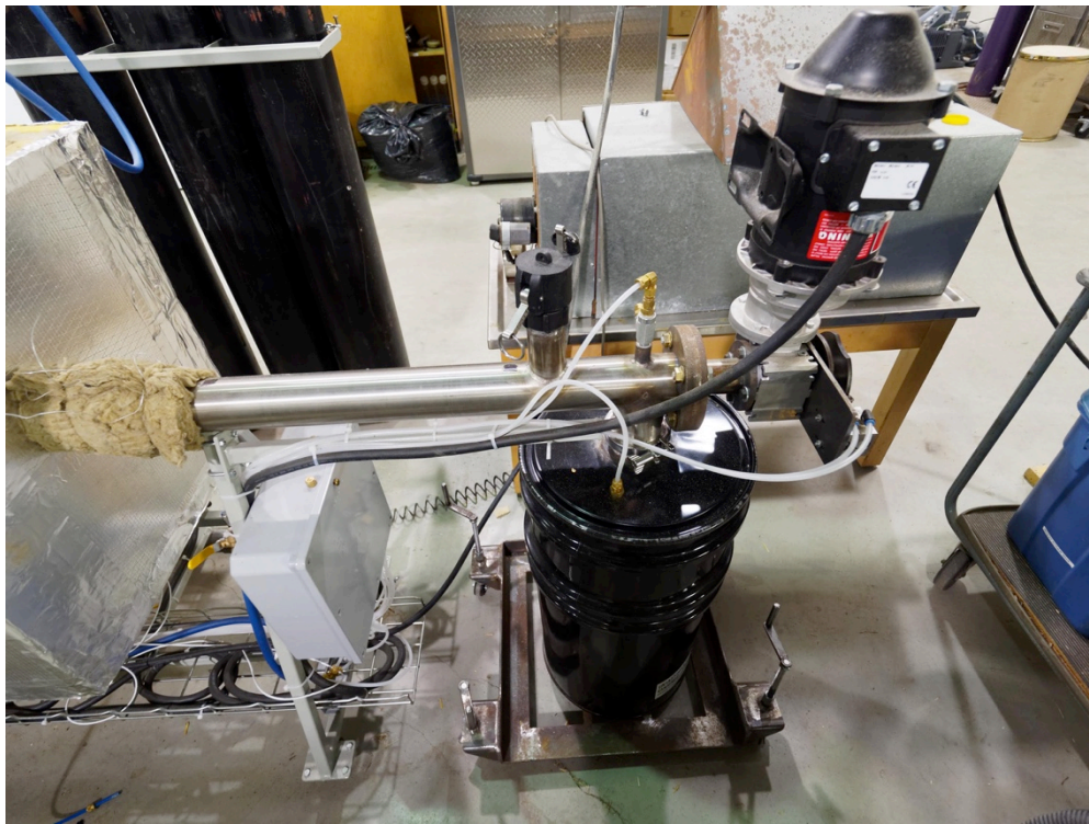
Figure A.3.15: Photograph of CTU pilot plant: Stage 2 discharge end, receiver and Motor 2.
