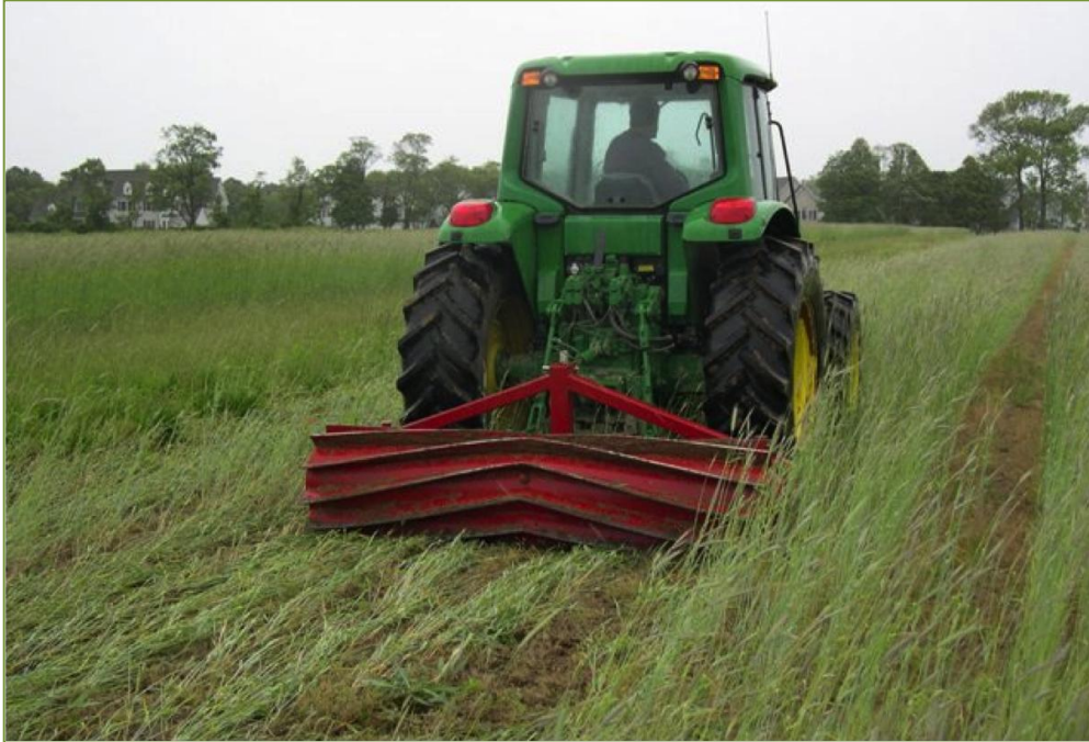
Figure 2.1 The roller-crimper is depicted terminating a cover crop. The chevron blades ‘crimp’ the stems, killing the plant tissue and laying the mulch on the soil. Source: http://www.nj.nrcs.usda.gov/about/2009Summary/2009_CTA.html
