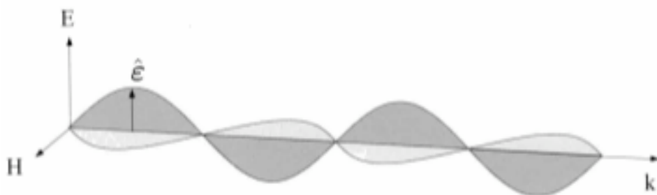
Figure 1.11 - Diagram of electric field vector perpendicular to vector of propagation, and orthogonality of electric (E) and magnetic (H) fields for linear polarization. (Figure adapted from J. Als-Nielsen and D. McMorrow, 2001)[29]
