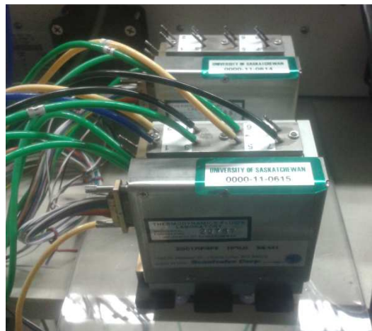
Figure 3.7: Scanivalve ZOC pressure scanner used for the seven-hole probe measurements.
