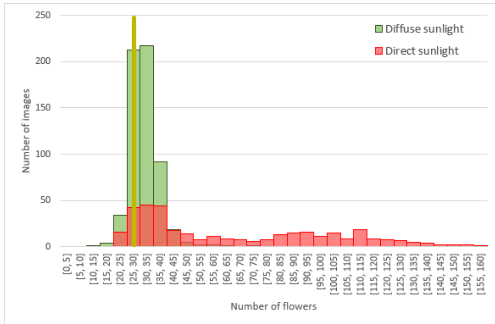
Figure 6.5: HoFC for manually-labeled diffuse sunlight (green) and direct sunlight (red) images from plot 1109 on day 1 from flowering. A gold vertical line marks the number of flowers in the plot determined by the ground truth.
