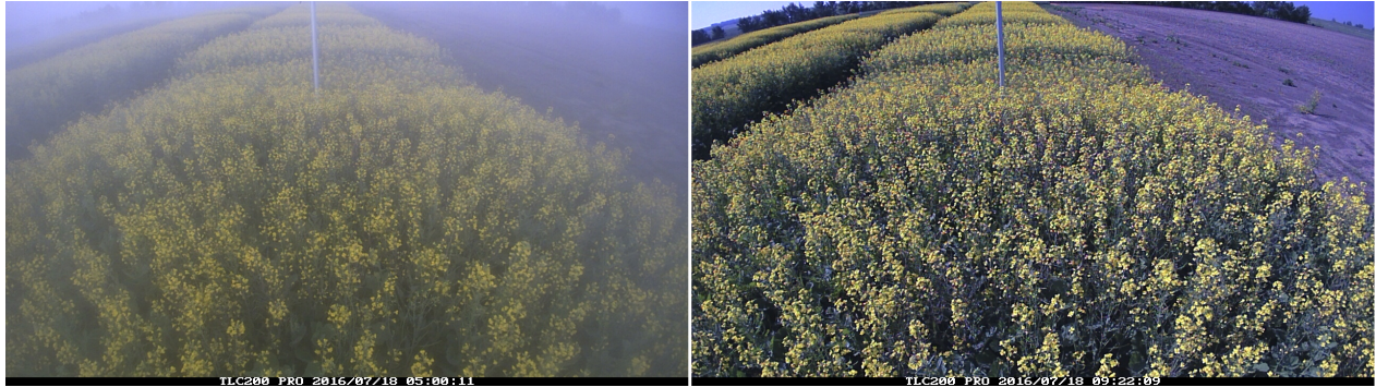
Figure 3.4: Comparison between an image with fog caused by condensation on the lens (left) and an image taken under normal conditions (right).
