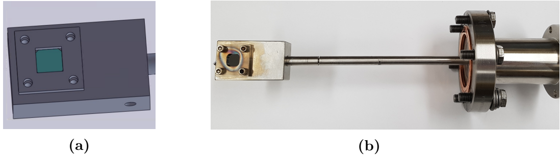
Figure 4.10: (a) SolidWorks drawing close-up of sample holder to show design details. (b) Picture of sample holder and translational vacuum feedthrough.
