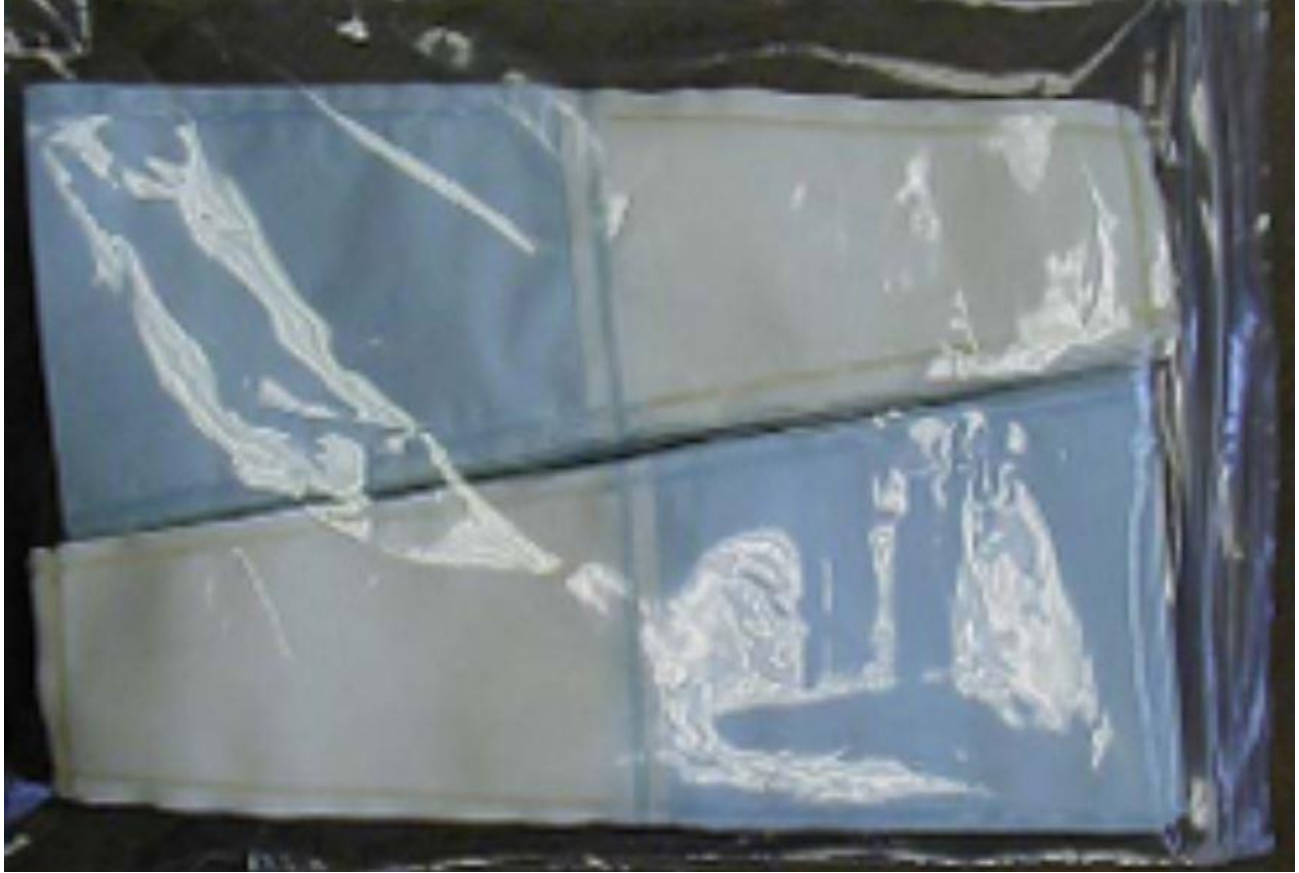
Figure 3–3: The X-Cell 100 Dust Sampling Sock used for dust sample collection (Source: Midwest Filtration LL website: http://www.midwestfiltration.com/dust-sampling.php ).
