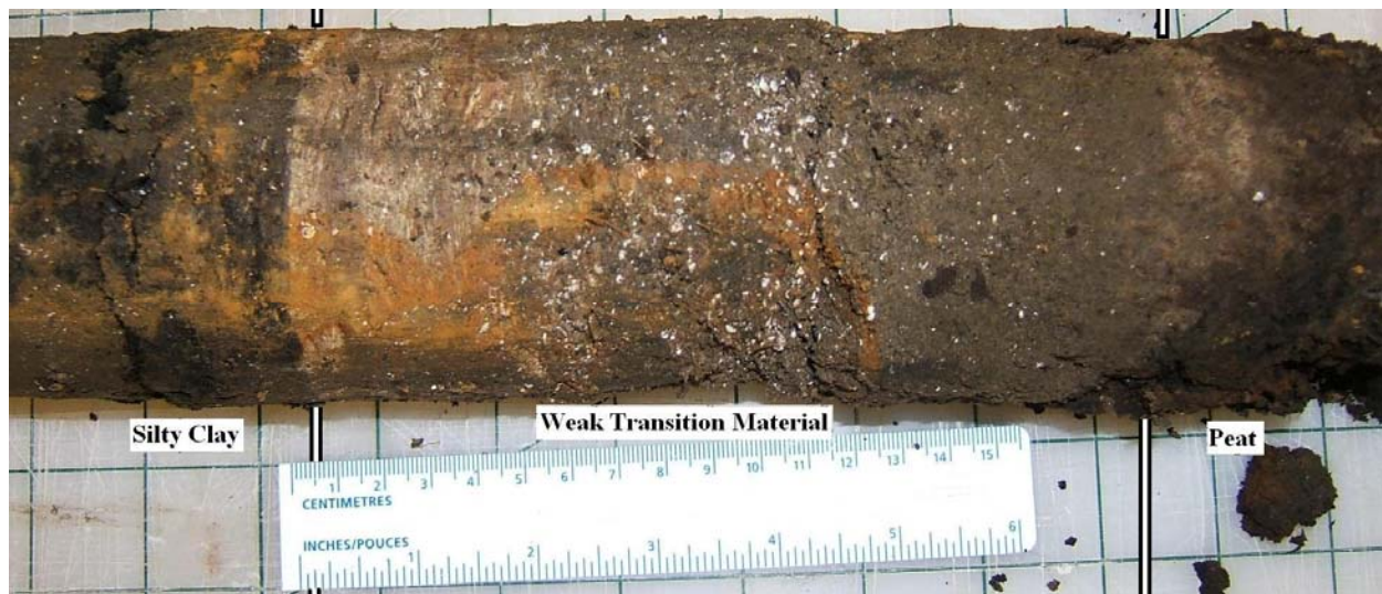
Figure 6.17: Pictures of the peat and silty clay interface and possible shear zone from Shelby tube sample taken at the under the centreline of the rail embankment at the Edson site.
