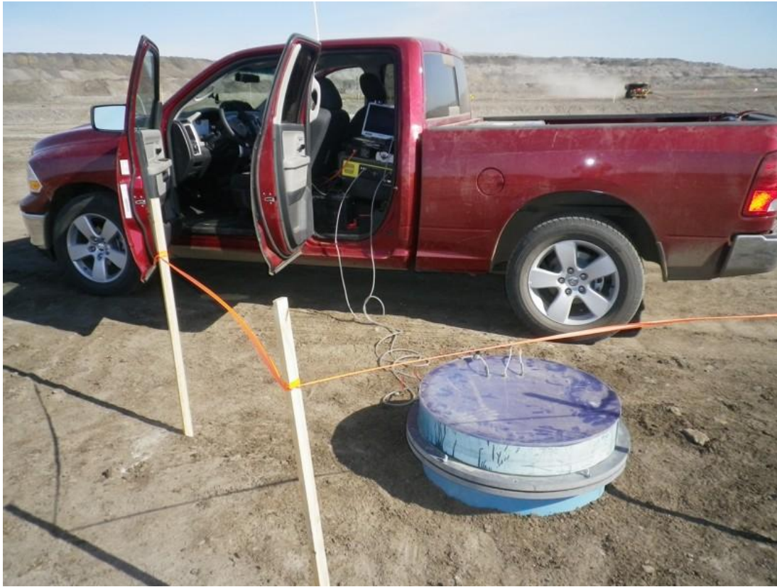
Photo 3.1. Gas flux measurement at Aurora Capping Study - facing NE
