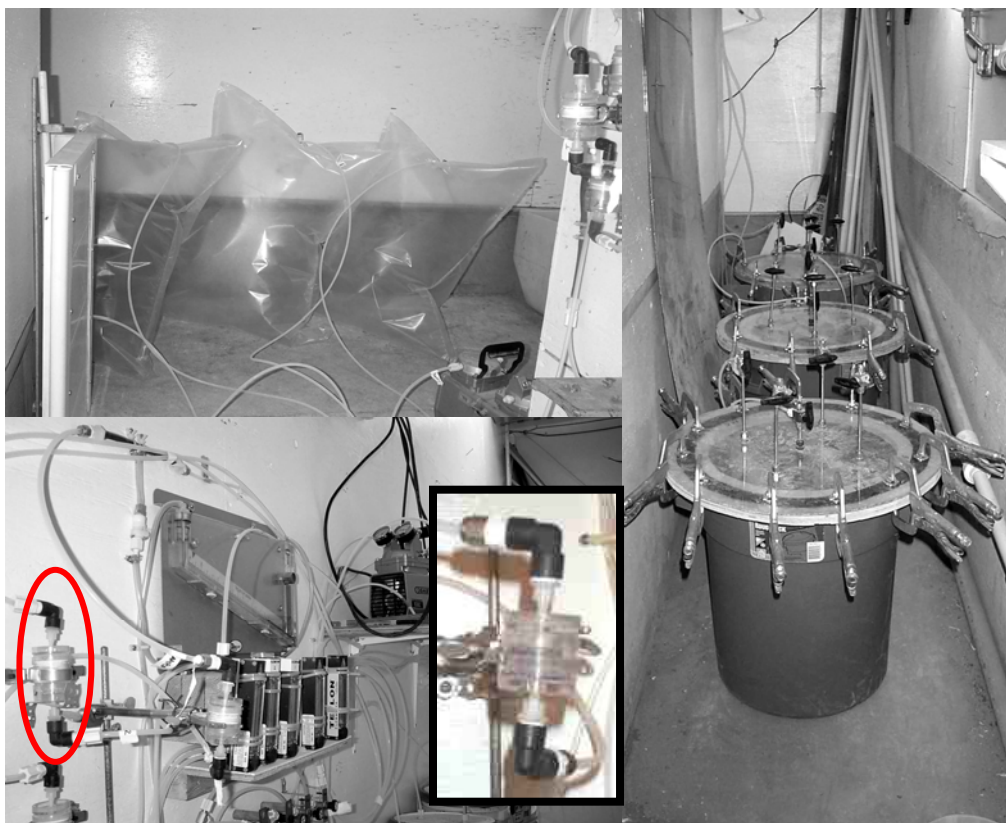
Figure 4.4.1 Photo of the actual set-up used for filtration method. Top: Input manure gas in 100-L bags. Bottom: Input gas was passed through cassette assembly with nanoparticles (inset); the gas flow rate and pressure drop across the filter was measured using flow meter and manometer, respectively. Right: Vacuum barrel used to collect filtered manure gas in sample bags.
