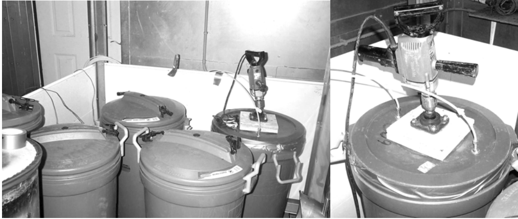
Figure 5.4.2 Photo of the actual set-up used for the mixing method. Manure slurry was mechanically agitated to mix the nanoparticles with the slurry and to generate gas during headspace gas analysis.
