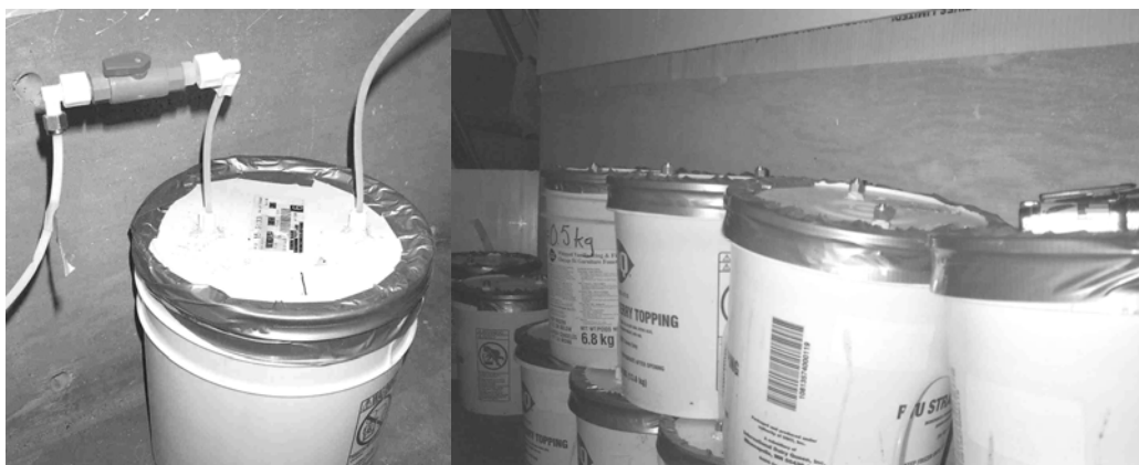
Figure 5.4.1 Four liters of manure was contained in 20-L pail covered with a lid. Gas was drawn from the headspace through a 1/4" opening and was recirculated back to the container after passing through the gas analyzers.
