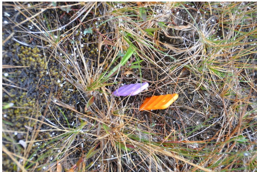
Figure 2. PRS probes installed in a minerotrophic bog.
