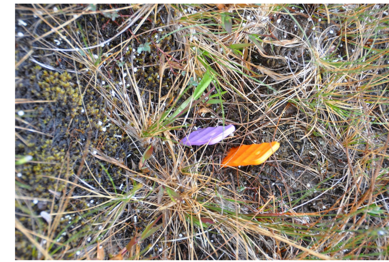
Figure 2. PRS probes installed in a minerotrophic bog.
