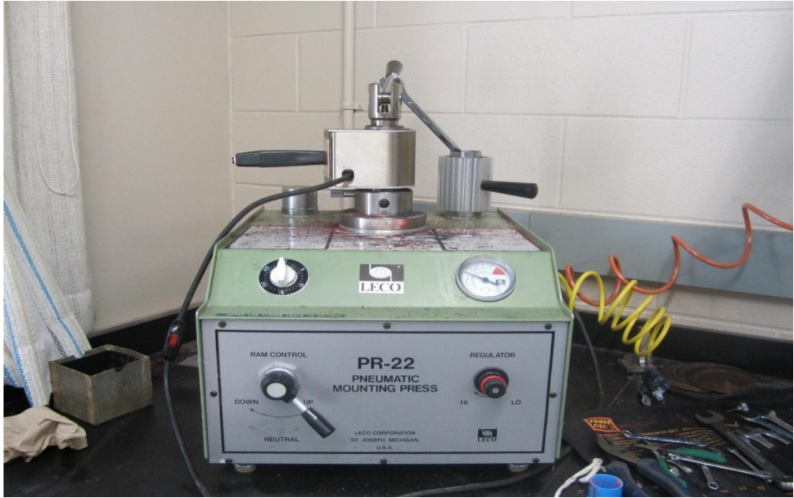
Figure 3.11. Photograph of pneumatic mounting press used for specimen mounting.
