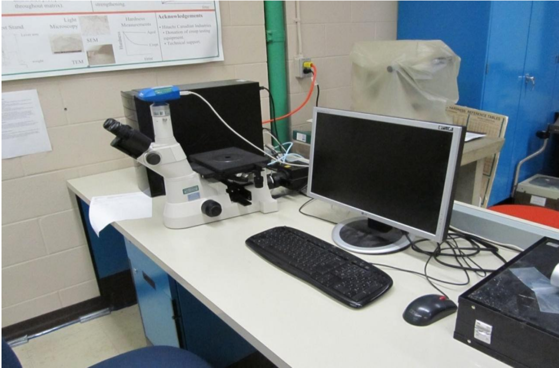
Figure 3.12. Photograph of the Nikon Eclipse MA 100 optical microscope used in this study.
