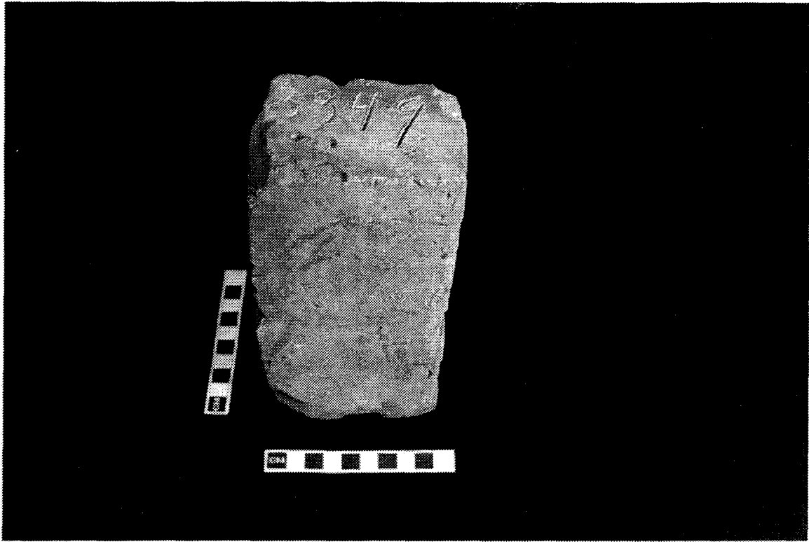
Figure 6.20 Bruno side-cut, non-textured brick with '3349' inscribed on end, before firing.
