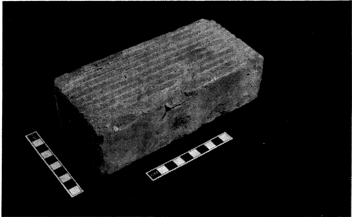
Figure 6.18 Bruno end-cut, ten-rib (one side) brick.
