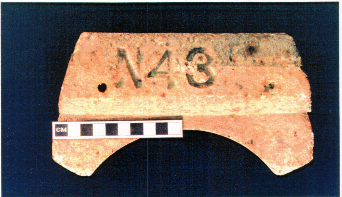
Figure B.10 Claybank hand-molded firebrick. Typical of the many unusual shapes made from the mid-1920s to 1989.
