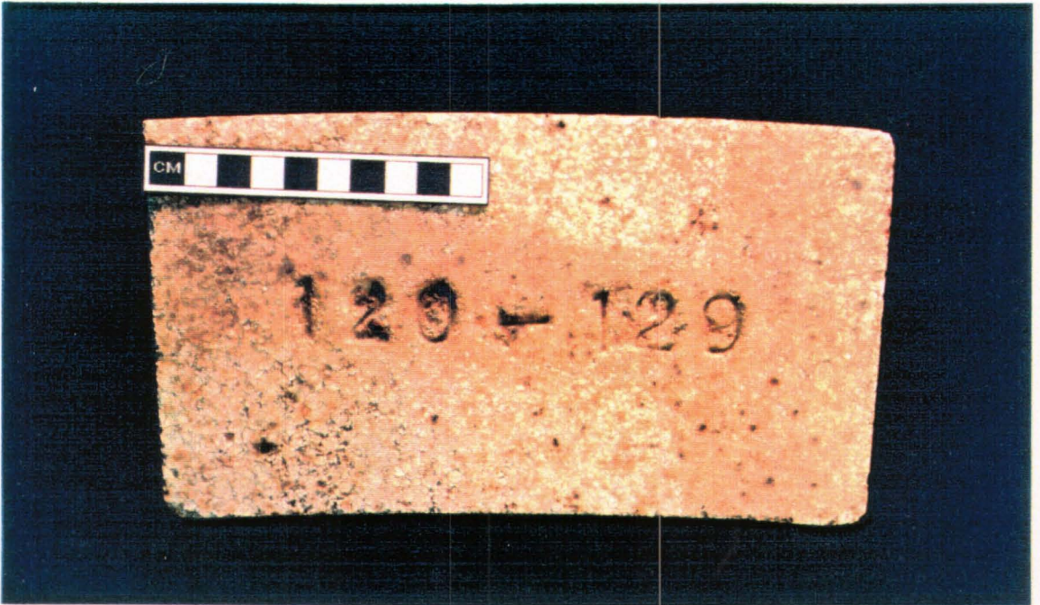
Figure B.11 Claybank circle firebrick, c.1980. (Numbers represent size of circle and are relatively standard among firebrick manufacturers).
