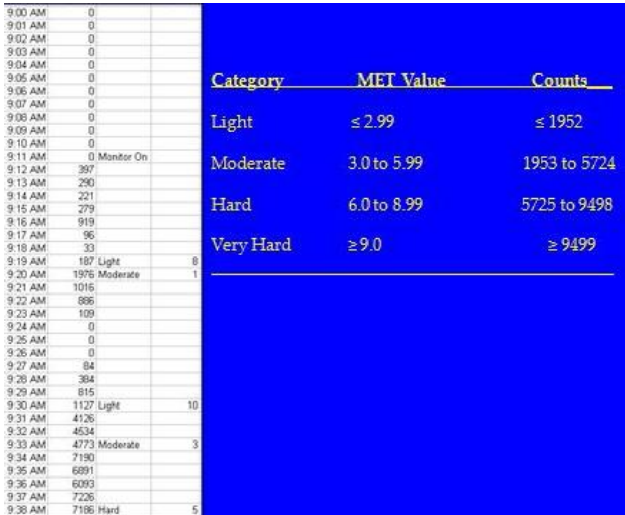
Figure 1.14. Tabular minute-by-minute accelerometer data complete with intensity categorization via the inlaid calibration chart.
